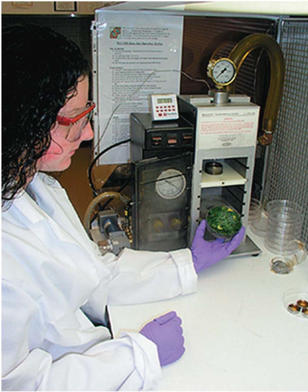
Figure 9.6 A gene gun, which can be used to insert DNA-coated “bullets” into a cell.
