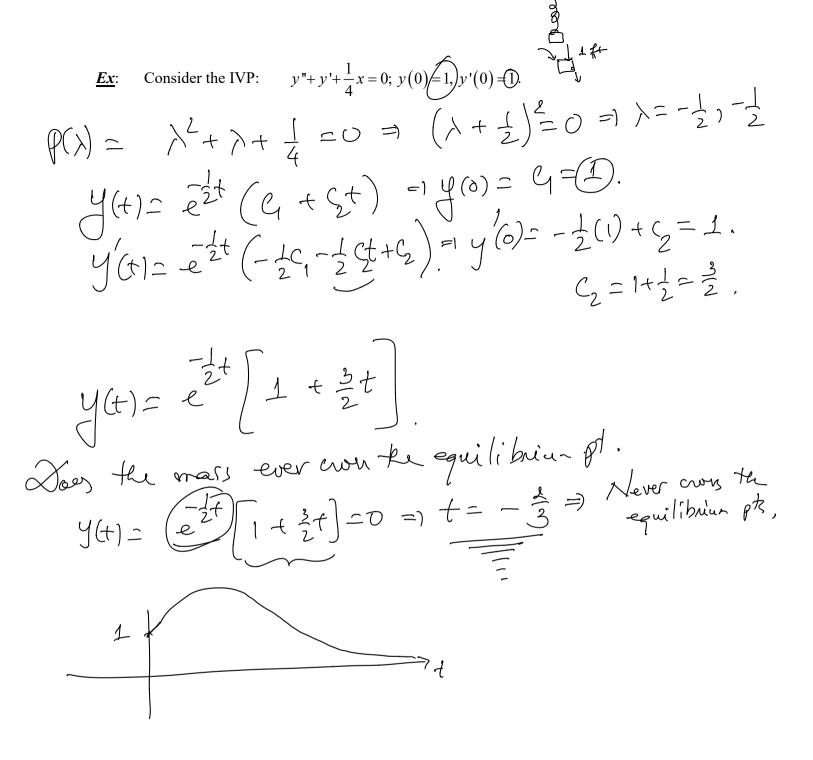
*Note*: The motion of a critically damped pendulum is similar to that of an Overdamped pendulum. In particular.
